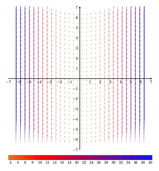
**Figure 1.** Vector field of dynamical system  $\dot{x}(t) = 1 + x^2(t)$
