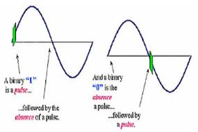
Fig. 1. Transmissions synchronized to zero crossing.
