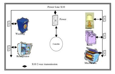
Fig. 4. Basic Configuration HCS interconnected with X10.
