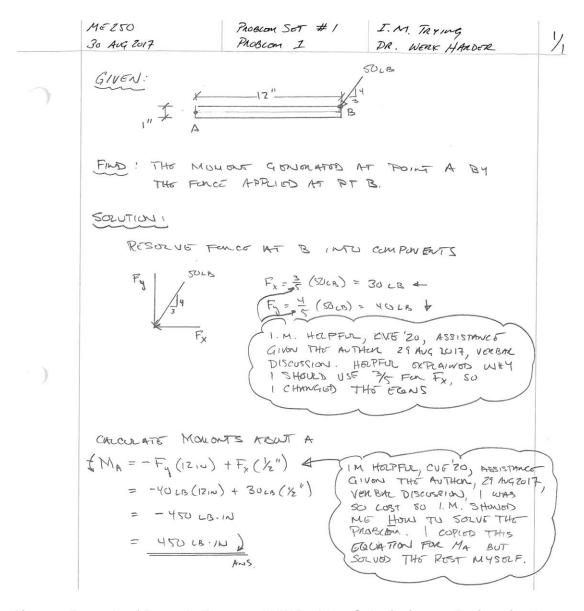
Figure 1 Example of Properly Formatted HW Problem Submission on Engineering Paper
