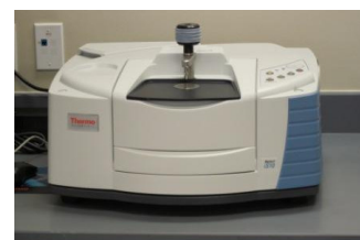
The Attenuated Total Reflectance (ATR) Infrared (IR) Spectrometer you will use to analyze some of the compounds made in this lab.
