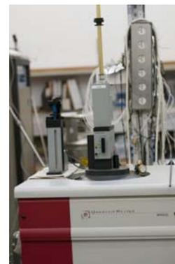
ASQUID (superconducting quantum interference device) is a very sensitive magnetometer used to measure very small amounts of magnetic material such as in metalloproteins. This image is taken from [https://superconductivity.biu.ac.il/files/superconductivity/imgs/gallery/lab\\_060311\\_02.jpg](https://superconductivity.biu.ac.il/files/superconductivity/imgs/gallery/lab_060311_02.jpg). (Accessed 08/16/20).
