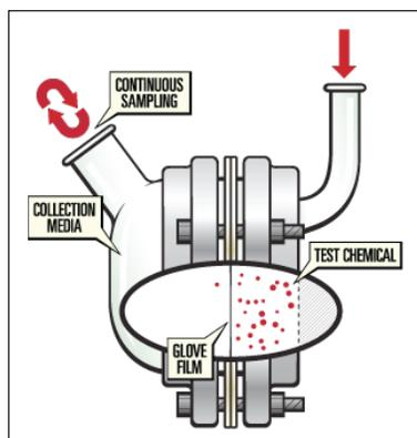
Permeation data is presented in two ways: Breakthrough time and Color code. Breakthrough times (min.) are the times observed from the start of the test to first detection of the chemical on the other side of the sample (see test chamber setup). These times represent how long a glove can be expected to provide effective permeation resistance when totally immersed in the test chemical.
