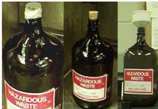
Improperly closed containers / container caps
