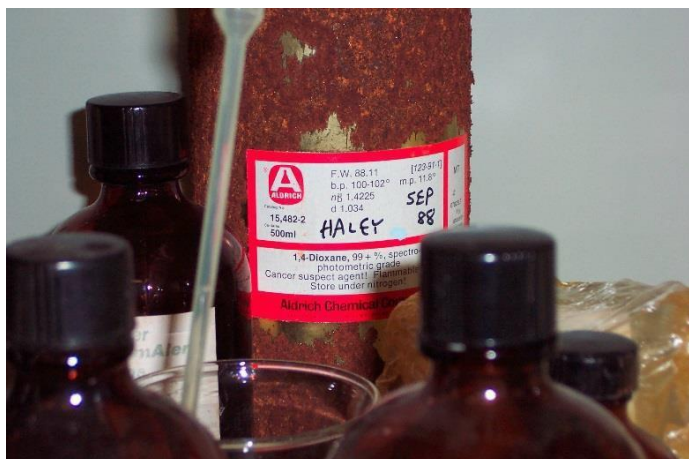
Chemical containers in poor condition from corrosion and crystal formation.
