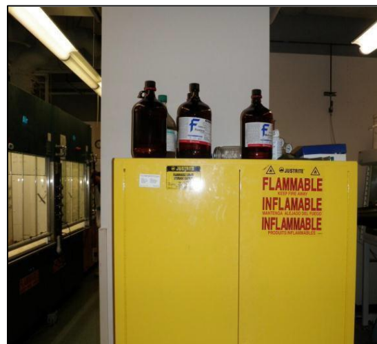
Improper storage of flammable chemicals above eye level
