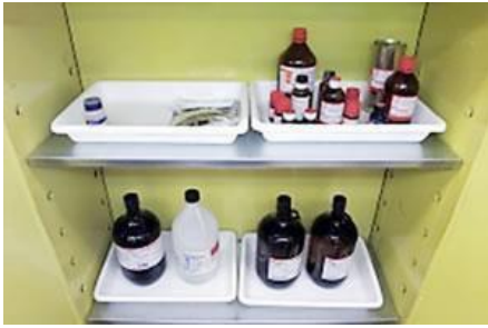
Shelves with secondary containment
