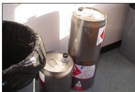
Improper storage of flammable chemicals
