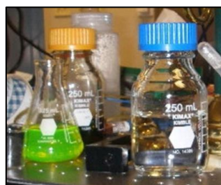
Improperly labeled secondary chemical containers
