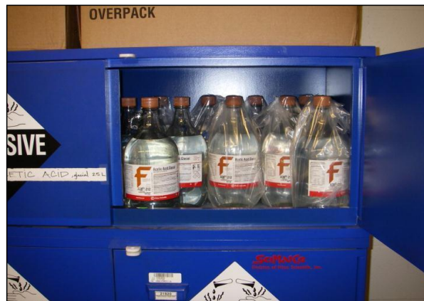
Acids stored in acid storage cabinet
