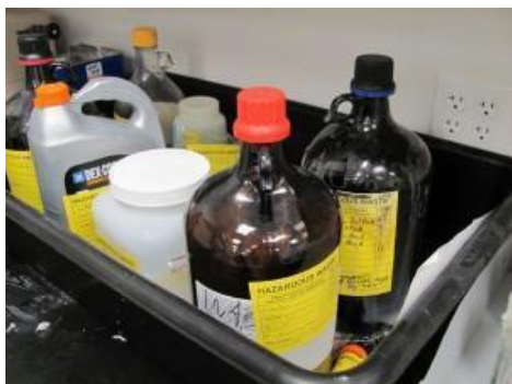
Properly closed waste containers
