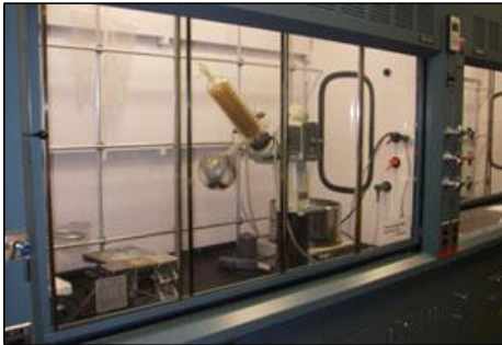
Proper use of a fume hood
