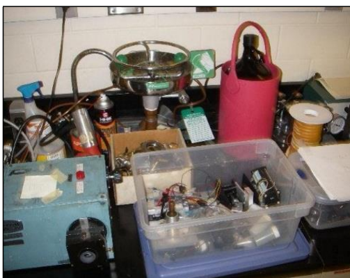
Emergency eyewash obstructed
