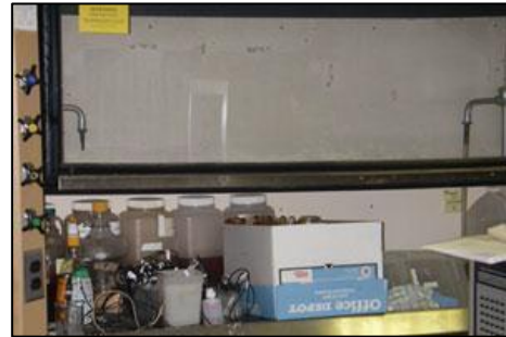
Improper storage in a fume hood
